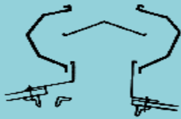
Existing roof with close ridge purlins
